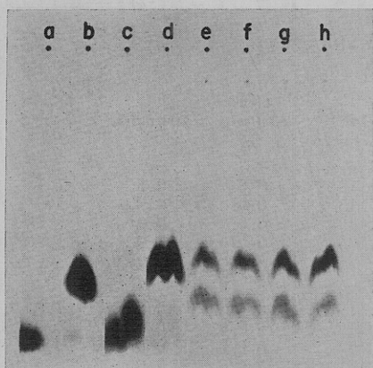
Figure 1. Chromatograms of extracts of lemon peel after applying isopropyl ester of 2,4-D labeled with C^{14} in the carboxyl position
