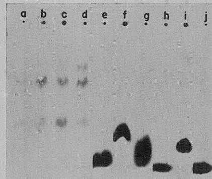
Figure 3. Chromatograms of extracts of lemon peel after applying isopropyl ester of 2,4-D labeled with C^{14} in the isopropyl group (1:3)
